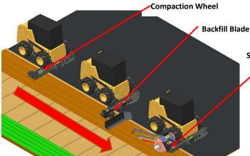
For ultimate efficiency, consider the SideTool Trenching Package. You only need one coupler to attach any number of SideTool attachments including the trencher, backfill-blade and compaction wheel.
