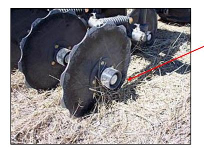
When an SCX crimper disc hits an object, it floats over or pivots around it, while the other discs remain firmly engaged with the soil. The disc pivoting action also allows for smoother, tighter turns for faster installation.
