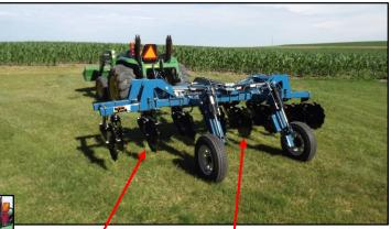
The SideTool SCX Straw Crimper's discs can pivot left and right and up and down independently, leaving a well-secured, even mulch installation
